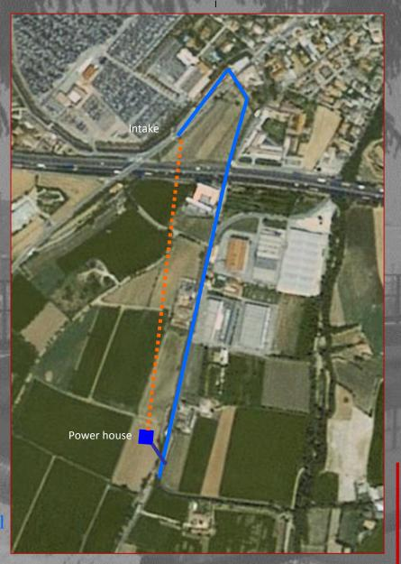
9.1 The part of the penstock realized with the jacking pipe technique
