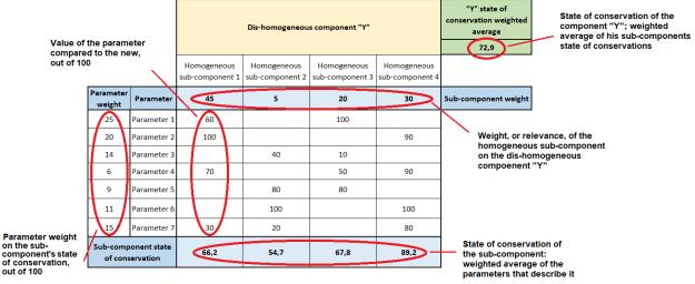
Fig. 2: State of conservation of the dis-homogeneous "Y" component
